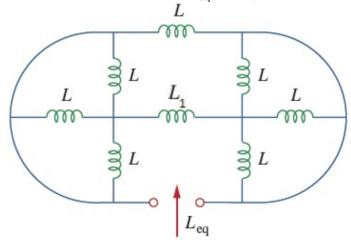
The equivalent inductance  $L_{eq}$  in the circuit is  $4.56 \pm 2\%$  H.
