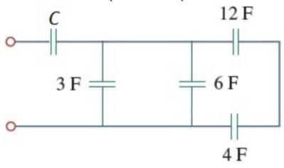
The equivalent capacitance is  $4.00 \pm 2\%$  F.
