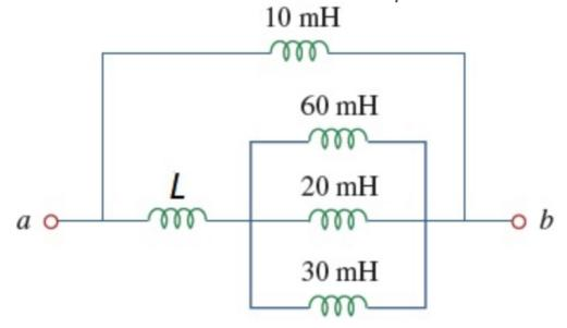
The equivalent inductance  $L_{eq}$  at terminals a-b of the circuit is  $7.222 \pm 2\%$  mH.
