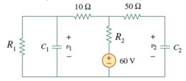
The voltage across the capacitors are  $v_1 = \begin{bmatrix} 42.58 \pm 2\% \\ \end{bmatrix}$  V and  $v_2 = \begin{bmatrix} 49.03 \pm 2\% \\ \end{bmatrix}$  V.
