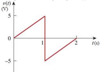
The inductor current for 0 < t < 1 s is  $i(t) = (89.29 \pm 2\%) t^2$  A
