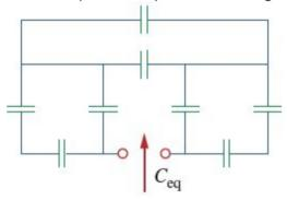
The equivalent capacitance is  $16.364 \pm 2\% \mu F$ .
