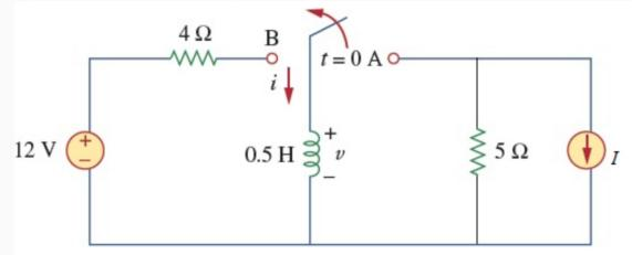
Find the voltage v(t) long after the switch is in position B.
