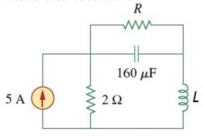
The value of R that will make the energy stored in the capacitor the same as that stored in the inductor under dc conditions is  $13.69 \pm 2\%$   $\Omega$ .
