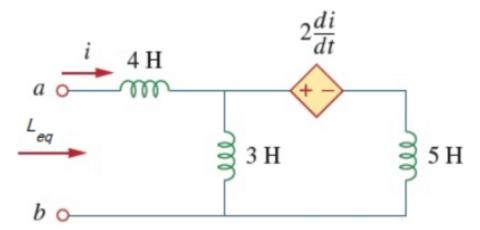
The equivalent inductance  $L_{eq}$  used to represent the inductive network is  $6.625 \pm 2\%$  H.
