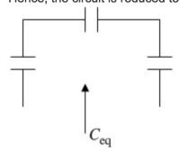
$$1/C_{eq} = ((1/45\,\mu\text{F}) + (1/45\,\mu\text{F}) + (1/60\,\mu\text{F})\,)$$
